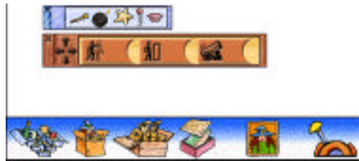
Fig. 1. This section of the Pathways screen shows two boxes that were opened from the icons in the control bar at the foot of the screen. The Toolbox at the top of the figure contains the following icons: a wand for copying; a bomb for deleting; a star for changing various settings of an object including its shape; a microphone for giving comments to objects and the mouth for speaking comments. The opened Stonesbox (below the Toolbox) is currently revealing some of the when stones. The when stones represent conditions such as “when I am touching”. The Stonesbox also contains do stones that represent actions such as “I jump” and behaviours that allow an object to be controlled by the mouse, joystick or keyboard. There are further icons in the control box to open a stored game, change the background, to create a new object in a game and to switch a game on or off.
